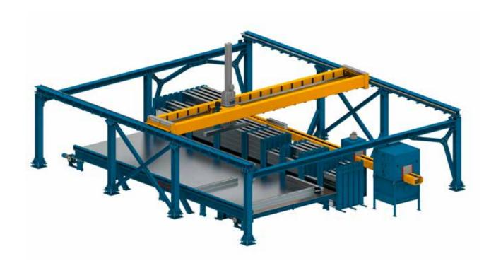
The large 2D plotter uses a specific program to import the file which will then be drawn on the pallet. The two-axis plotter draws the boundary lines of the panel and the various integrated parts. The master computer on which the application software will be loaded will manage the files created by the technical office. All post processes will be viewable on the various HMI panels located along the production line.
