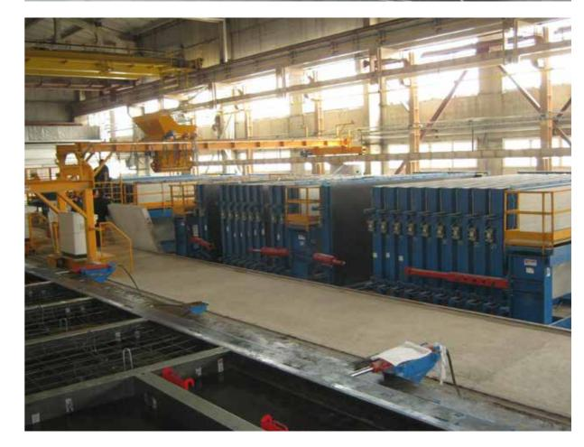
The vertical demoulding of the product is very rapid, thanks to the automatic movement of the lateral containment bases. Each pocket can be opened up to 2 m/6,5 ft for setting and disarming operations (according to the customer's specific request). Thus to allow, operator working in total safel and comfort.
