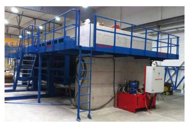
High-tech formworks for the production of small and large prefabricated elements:
