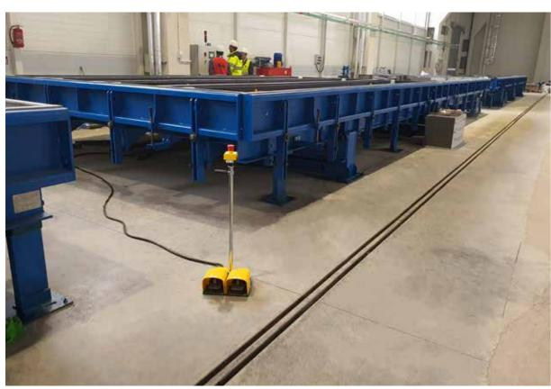
The long-lines, suitable to manufacture prestressed elements, are equipped with fixed and mobile pull heads. The mobile heads are supplied with hydraulic relaxation cylinders. The tables do not need special foundations to be placed, but simply a 350 mm/13,7" thick industrial floor. The stressing heads are equipped with protective cages to protect from strands.
