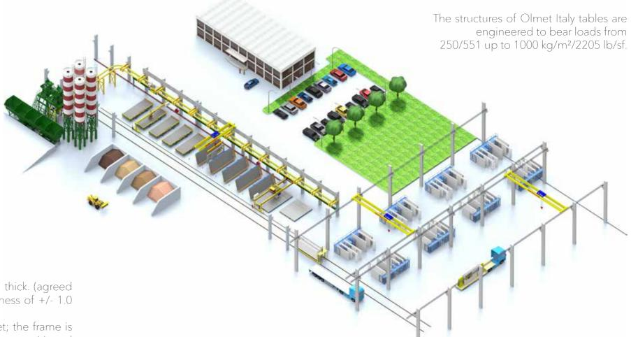
The casting steel sheets are of the highest quality, usually 10 mm/0,4" thick. (agreed with customer); they are welded on the frame ensuring a surface flatness of +/- 1.0 mm/0,04". per meter.
