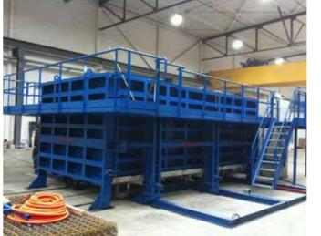
with a special oleodynamic station suitable for the control of 4 + 4 telescopic cylinders for lifting.
