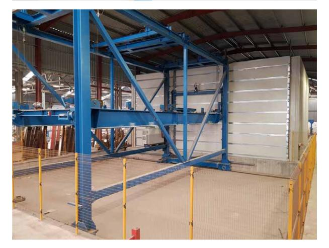
The flat elements produced are floors, solid walls, double walls, sandwich walls, but also special large format elements. The innovation of this system consists in organizing production on preparation stations manned by one or more employees. This system provides significant advantages for companies, which will have to standardize both the production process, which the component parts, with positive impacts in terms of reduction of production times and costs.
