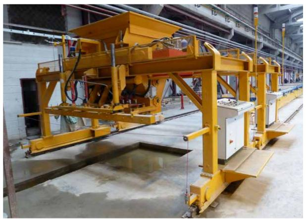
Independent hydraulic cylinders allow the opening and closing of the outputs, single or multiple, through proportional valves. The machine can be managed manually via remote control with a single operator, or controlled through specific software.
