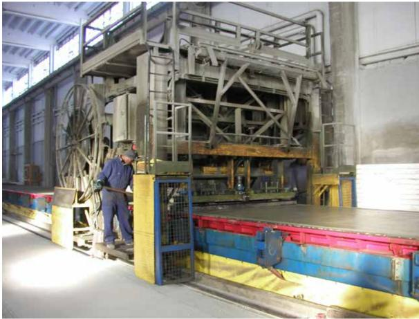
The heating system, to accelerate the concrete curing is composed of longitudinal pipes connected to a coil; it is possible to use steam, hot water, diathermic oil, or electrical resistances as a thermal agent.
