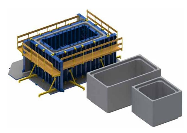
The side elements can be removed, for the demoulding of the concrete element, by mechanical handling with the overhead travelling crane; alternatively, there is the possibility to move them with double-acting hydraulic cylinders.
