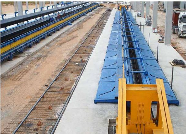
The formworks according to their size, therefore according to the size of the beam, are manufactured in 6 mm/0,2" - 8 mm/0,3" - 10 mm/0,4" casting side plates. They are always complete with:
